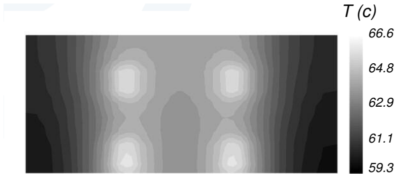
Figure 5: Reduced temperature differences with optimised heat source placement (simulated)
