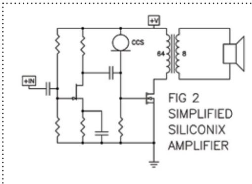
driven by a J106 JFET shown in Figure 2. He went on to simplify this circuit by eliminating the input JFET, driving the Gate of the power MOSFET directly (Figure 3).
