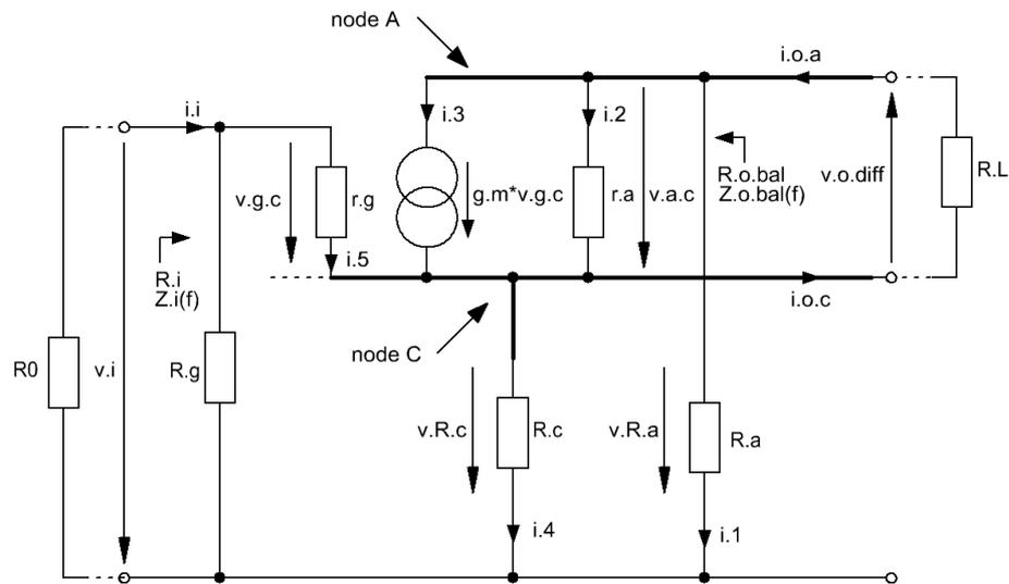
Fig. 1 Equivalent circuit of a CPS
