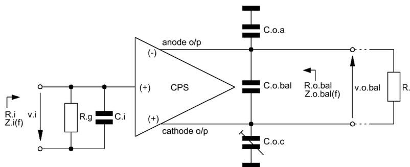
Fig. 3 Principal gain-stage set-up with output capacitances
