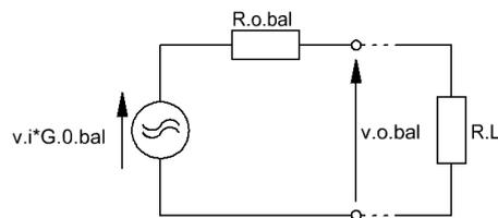
Fig. 2 Simplified equivalent circuit of Fig. 1
