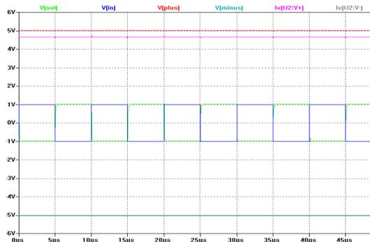
Figure 6.3(L): LT LT1354 model, taking a constant current from each rail (but not the same value)
