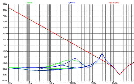
Figure 2.5(L): rail impedance as we increase the regulator output cap from 2.2uF up to 2200uF, decade steps. This is with the noise bypass caps.
