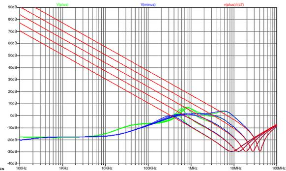
Figure 2.4(R): impedance plots of the supply rails with tantalum capacitors. Contrast with figure 1.2 in part 1
