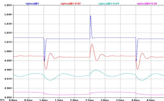
Figure 2.8(R): the response of figure 2.7 to the 0-10mA 333Hz square wave. Talk about ringing!
