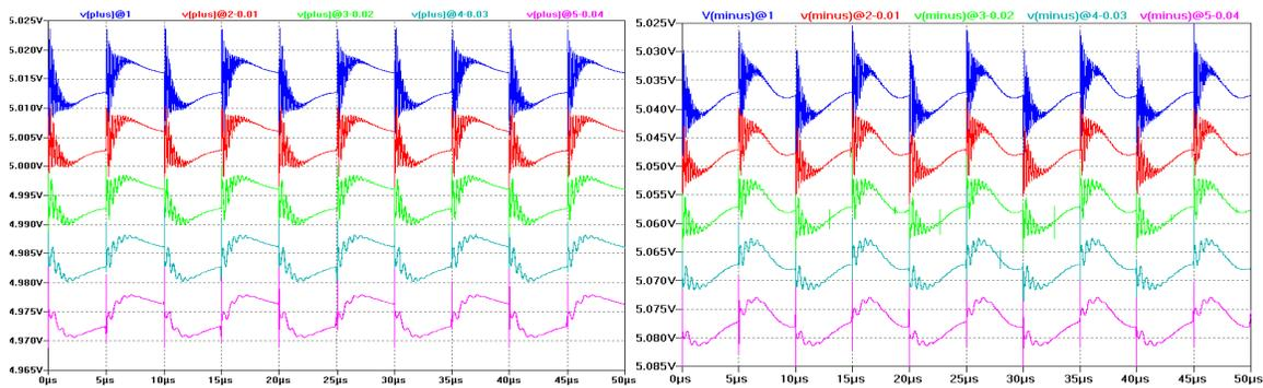
Figure 2.1(L): pinging the positive rail with 100kHz 0 to +10mA square wave, 5mV/div, traces spread by 10mV
