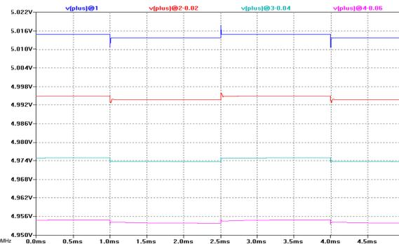
Figure 2.6(R): voltage on the rails when 0-10mA squarewave at 333Hz is applied. 2.2uF top, 2200uF bottom.
