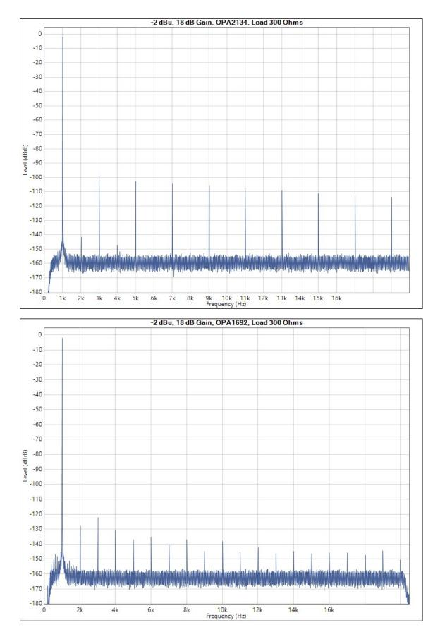
Please note that due to internal serial resistors in the AR, the real output load was a total of 700  $\Omega$  for this measurement. First pic details an OPA2134, second pic an OPA1692. Unfair comparison, yes, but it just shows how easy it becomes to verify manufacturer specs, and to see the real-world performance with the levels/impedances that one needs in a design. Just plug it into the AR!
