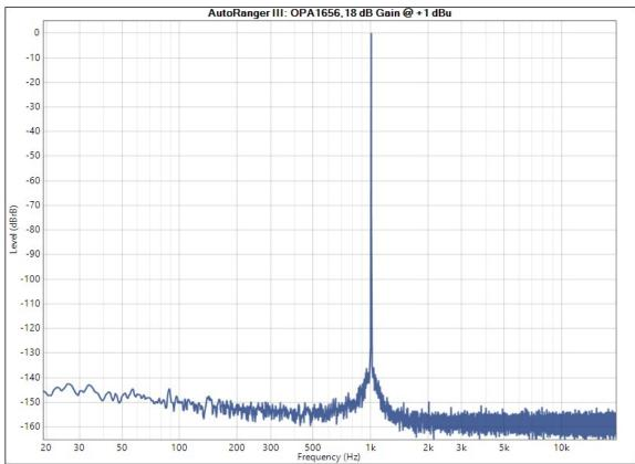
Setting the AP to 300  $\Omega$  input impedance puts a hefty load on the opamp in the AR. Differences here are quite big. Two examples of +16 dBu balanced output level, so every opamp stage processes +10 dBu only.
