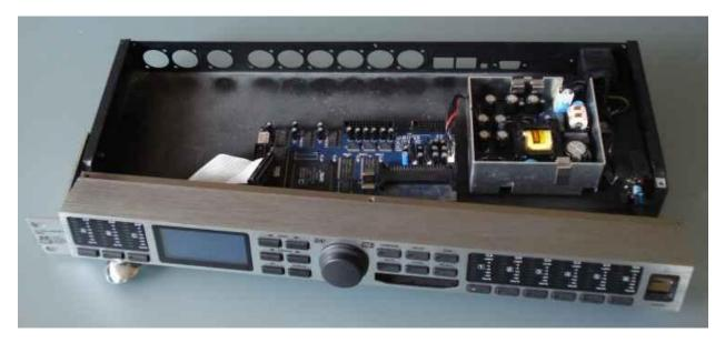
There is an off-board replacement XLR connectors in the kit for the digital input. Mount this connector now in the 'A' input slot using the original screws. (The analog input connectors will be on the new board and be mounted at positions 'B' and 'C'). When we get to the testing part, you need this input to get some signal into the unit.
