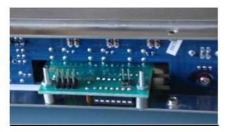
Next, carefully mount the display/control board with the included 2.5mm hardware and the 8mm stand-offs. It should look like the pic to the left. The display should just touch the Plexiglass window at the front. Double-check that the board is not bend or anything and that there are no obvious shorts or mechanical problems. Note the plastic sheets and the reverse-mounted J1, J7.
