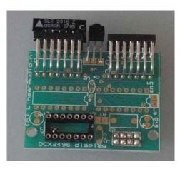
Stuffing the control and display board.
