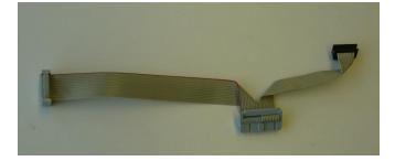
Now fold the short end over the middle connector and put on the cable clamp as shown in the pic at left. This completes the power supply cable.
