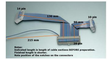
If you have a multimeter, it's a good idea to check for continuity between like pins and the absence of shorts between different pins. And finally, the signal cable. The best way is to start with the main 2\*13 pin connector, mounted with the notch as shown.
