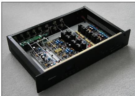
PHOTO 4: An LBAudio/Borbely Audio All-FET line-amp on Teflon PCBs, using Welborne Labs' input selector and attenuator with remote control. (Courtesy LBAudio.)
