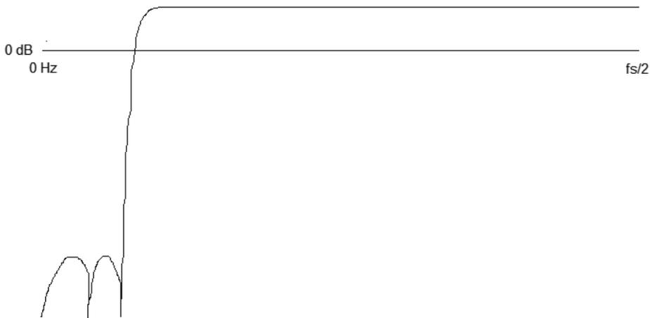
Figure 5 Sketch of a noise transfer function, magnitude in dB versus frequency on a linear scale. According to the Gerzon-Craven noise shaping theorem, the area below the 0 dB line can not be greater than the area above the 0 dB line.
