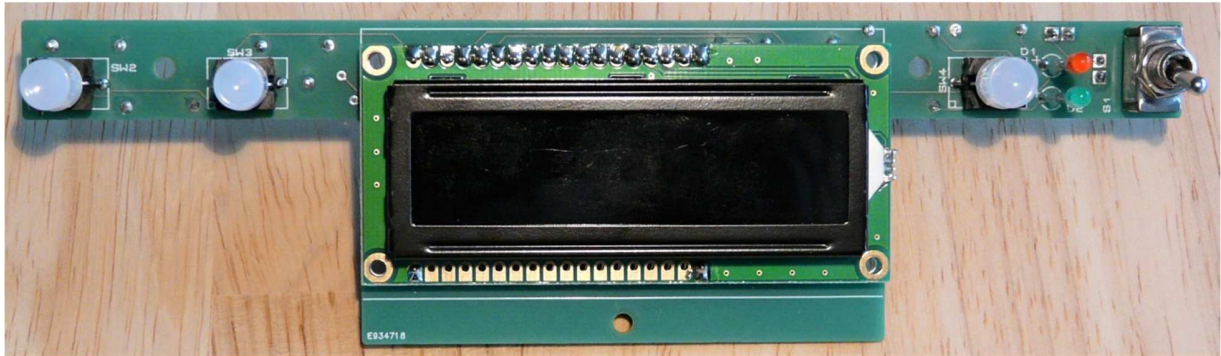
Figure 5 – completed front side display & control board
